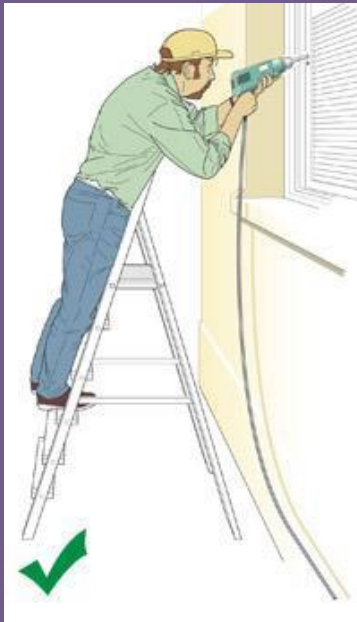
Correct - steps facing work activity
